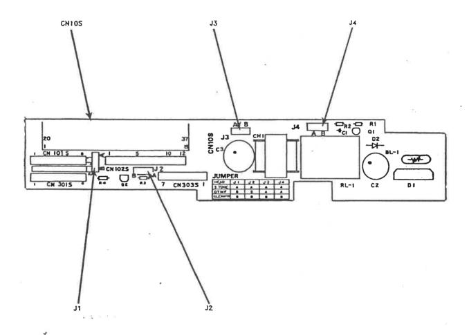
Figure 7-1. Jumper Positions on Terminal Unit PCB
